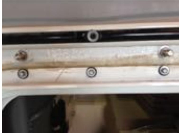
step thirteen: using a small screw driver, lever up the clip (do not remove it) and push with your hand, to pop the strut onto the ball brackets.... done!
